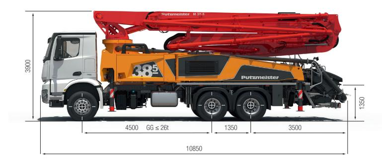
Note: Standard version. Dimensions and weights depend on truck, pump model and equipment. Dimensions in mm, MAN TGS 26.400. For illustration only.
